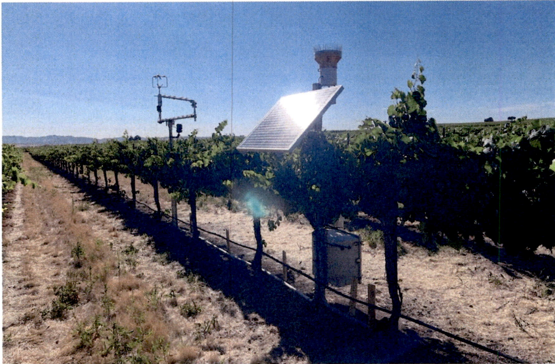
Figure 1 – An example Land IQ evapotranspiration station, viewed from the southeast, located in an east-west oriented vineyard.
