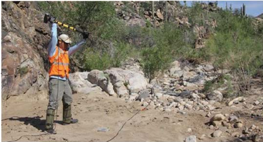
Seismic refraction surveying
